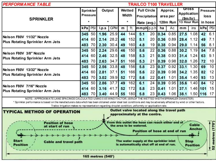
**Hose Size:** 38mm (1<sup>1</sup>/<sub>2</sub>") x 67 metres (220') Hose **Cable Length:** 120 metres (394')
